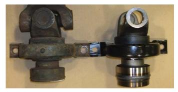
The factory original driveshafts found on various 2003-2006 Chevrolet and GMC G3500 Express Models have a non-replaceable center support bearing. With the Rockford Kit you are able to cut the Original assemblies apart 1/4" below the friction weld and replace the Yoke and Center Support Bearing.
